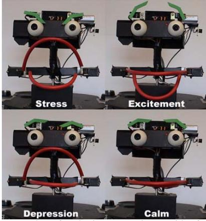
Figure 3. Example of robotic expressions with four assigned feature-level emotion labels.
