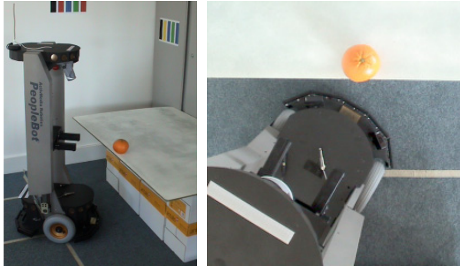
Figure 1: The PeopleBot robot during the docking manoeuvre. On the left are visible the camera pointing downward (mounted underneath the top plate) and the black grippers. Right, the scenario from above. The black grippers are hardly to be seen over the dark robot's base; a fraction of the camera can be seen bright.
