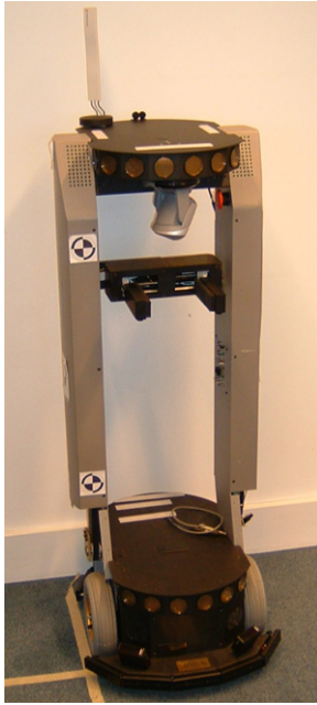
Fig. 5. PeopleBot used as the base for the acoustic model.
