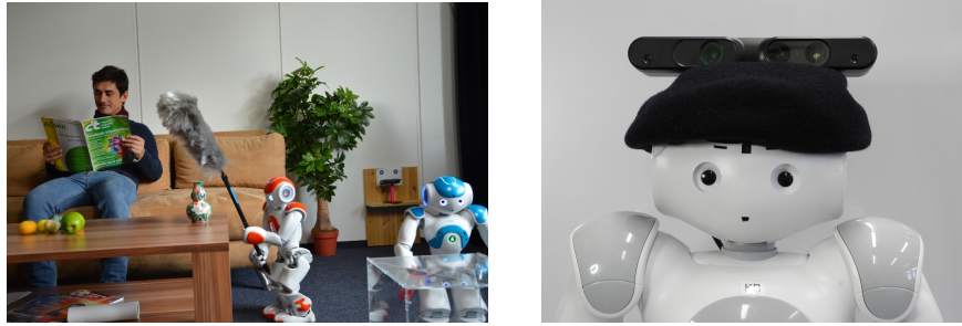
Fig. 1. (Left) Final scenario to be used and (Right) NAO robot with RGB-D device.
