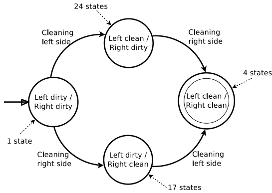
Fig. 8. Given that the cup is on the left side, there are two feasible paths for reaching the final state from the initial state. The lower path would include 17 possible different states and consists of cleaning first the empty side of the table, and then moving the cup in order to clean the second side. The upper path would include 24 possible different states and consists of moving the cup first to the empty side and cleaning this side, and after that returning the cup to its original side for cleaning the second one. In each case, the final state is reached involving different numbers of intermediate states. The ending sequence of the task contains four states in which the robot returns its hand to the home location and drops the sponge.
