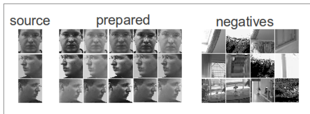
Fig. 1. Samples of the training set. Only three source images were used (left), afterwards we created additional images with different randomly changed width, height, rotation and gamma corrections, finally reaching 35 images per pose (middle). On the right are samples of randomly cropped negatives of landscape, offices and flat images taken from the internet.
