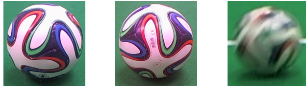
Fig. 1. One of the balls currently used in Robocup. The white color of the ball is almost identical compared to the color of the goal posts and the endlines. In the center image one can see the overemphasized red channel; this happens occasionally with our robot’s camera and the lighting in our laboratory. The left and center images show non-moving balls with a distance of 0.5 meters to the robot. The right image shows a moving ball with a distance of 1.0 meter to the robot.
