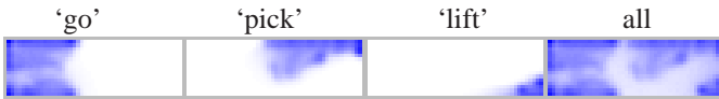
Fig. 5. Trained weights W^{td} to four selected language units of the student robot. Each rectangle denotes the hidden area, dark are strong connections from the corresponding regions. Each of the three first units is active only at one input, denoted above. The rightmost unit is active by all language words.
