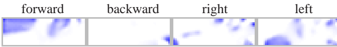
Fig. 6. The trained weights W^{td} to the four motor units of the student robot. As in Fig. 5 the regions from which strong connections originate in the hidden area are depicted dark.
