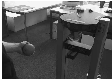
Fig. 2. The MIRA recognising and tracking an orange with its camera.
