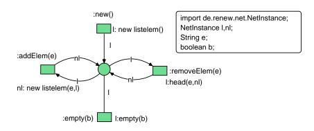
Fig. 3. A list implementation using the net instances of Fig. 2
