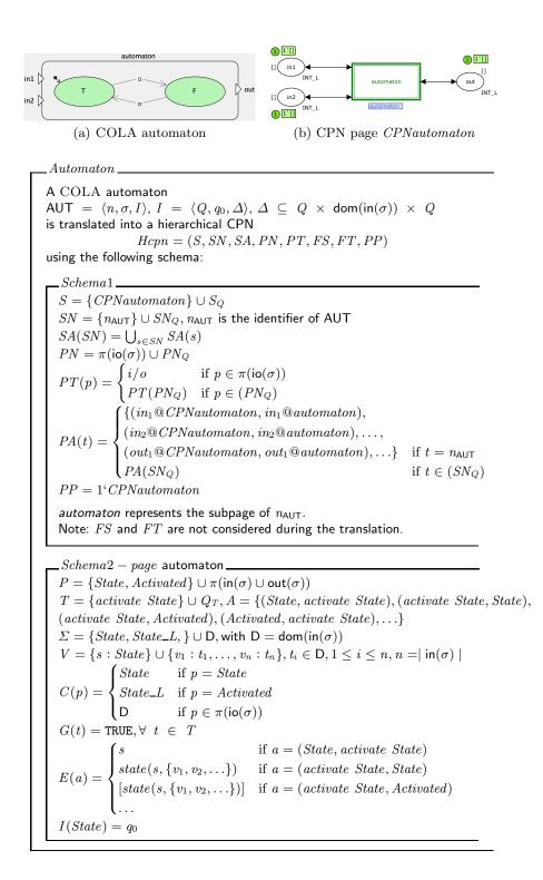
Fig. 6. Exemplary (a) COLA automaton with two states and (b) its translation, and the translation schema.
