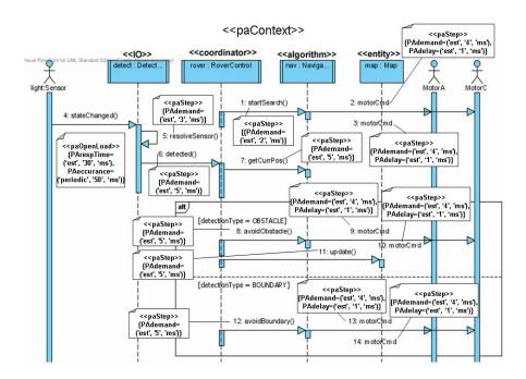
Fig. 4. Robot controller PSM interaction diagram
