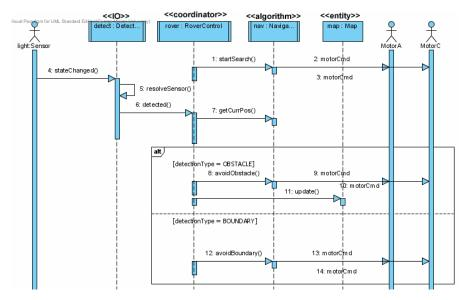
Fig. 3. Robot controller PIM interaction diagram
