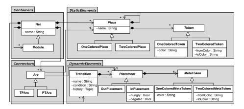
Fig. 2. The Transformation Net Metamodel
