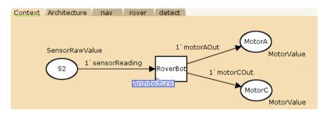
Fig. 5. Robot controller context level CPN
