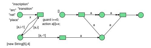
Fig. 4. Example of flexible arcs
