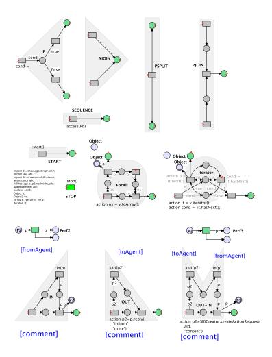
Fig. 1. MULAN Protocol Net Components
