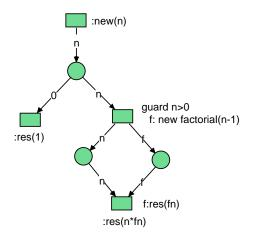
Fig. 9. Recursive net for calculating factorials
