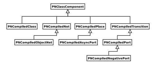
Fig. 6. The inheritance hierarchy of the classes of the OOPN class metaobjects.
