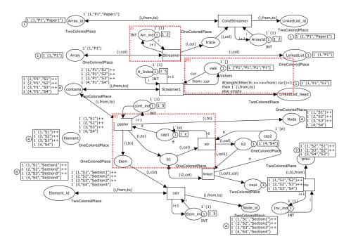
Fig. 8. Array2LinkedList using CPN
