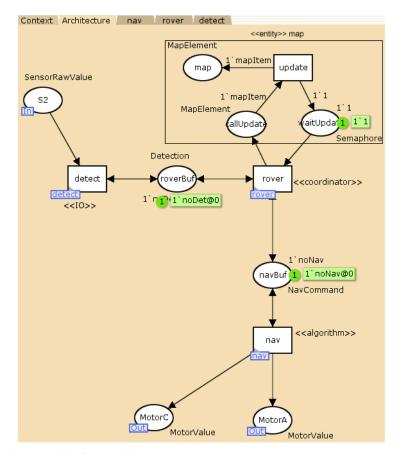
Fig. 6. Robot controller CPN architecture
