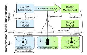
Fig. 1. Conceptual Architecture of Transformation Nets
