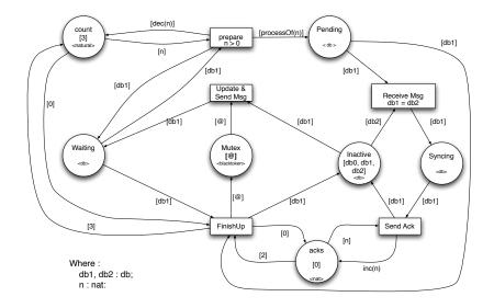
Fig. 1. Distributed database Algebraic Petri Net model
