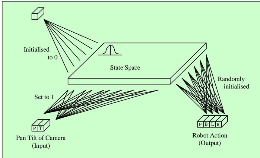
Figure 7 - Architecture used for the navigation control unit from Figure 5
