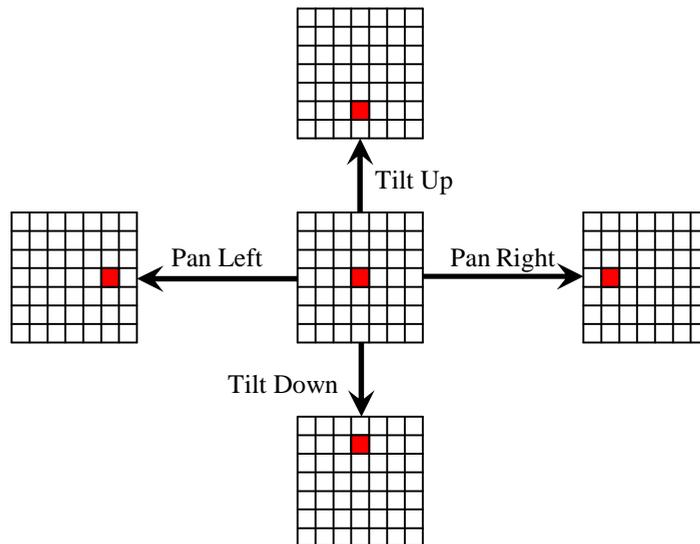
Figure 9 - Simplified effects of camera movement on the location of the landmark in the image. The red square represents the landmark
