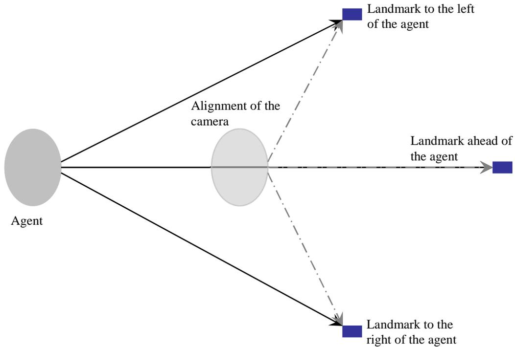
Figure 10 – Diagram to show the effects on the orientation of the robotic camera as the robot moves in a forward direction relative to the landmark. It can be seen that if the landmark is to the left of the robot, moving forward causes the camera to pan to the right. If the landmark is to the right, moving the robot forward causes the camera to pan to the left. Finally if the landmark is straight ahead the pan angle does not change.
