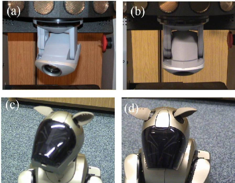
Figure 3 - Example of the camera alignments for the two test robots. (a) and (c) show the cameras of the two robots pointing at a landmark to the front right of the robots. (b) and (d) show the cameras of the two robots pointing at a landmark directly ahead and at the base of the robots.
