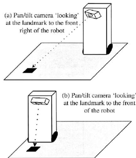
Figure 4 – Example of different camera alignments (a) position of the camera with the landmark located to the front right of the robot and (b) position of the camera when the robot is at the landmark.
