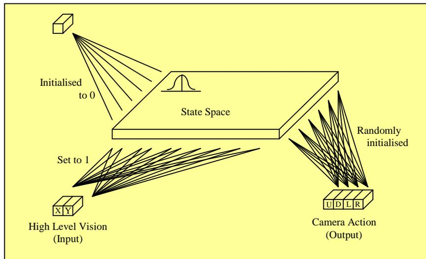
Figure 6 - Architecture used for the camera control unit from Figure 5
