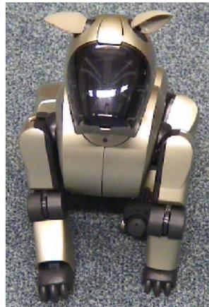
Figure 2 - Sony Aibo robotic dog
