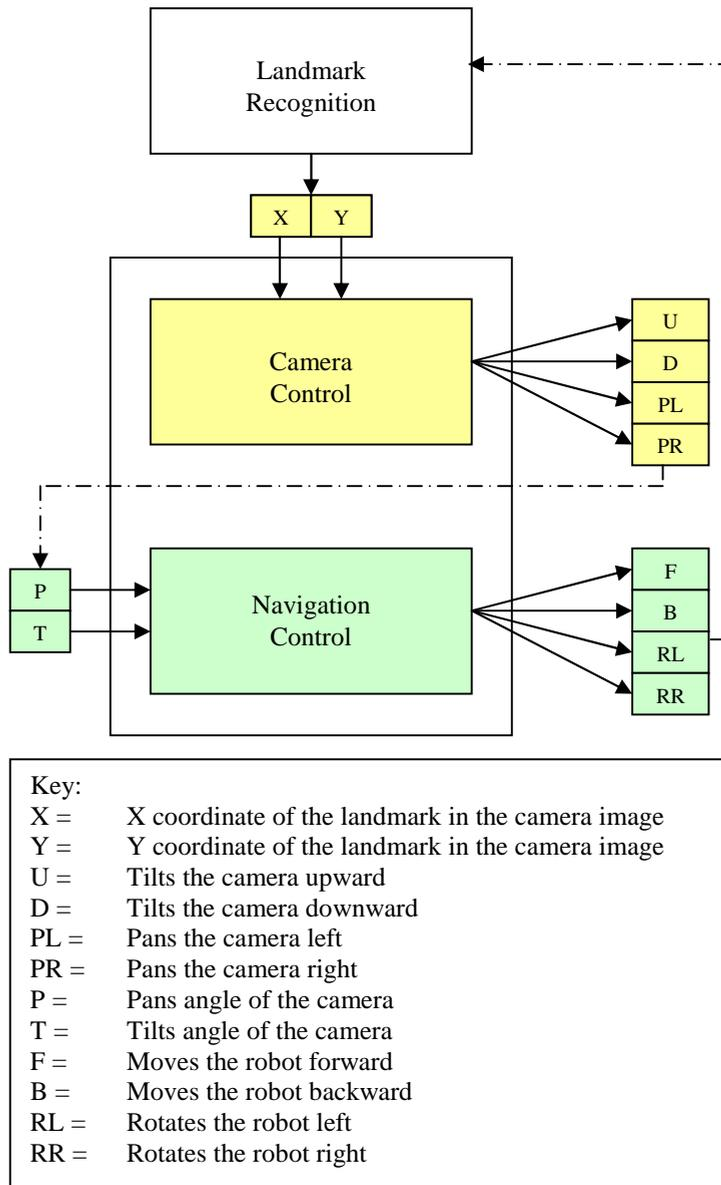
Figure 5 - Overview of the MAC Architecture. The core components are the 2 control units, which support platform independency. Only the landmark recognition may need altering slightly for each platform.
