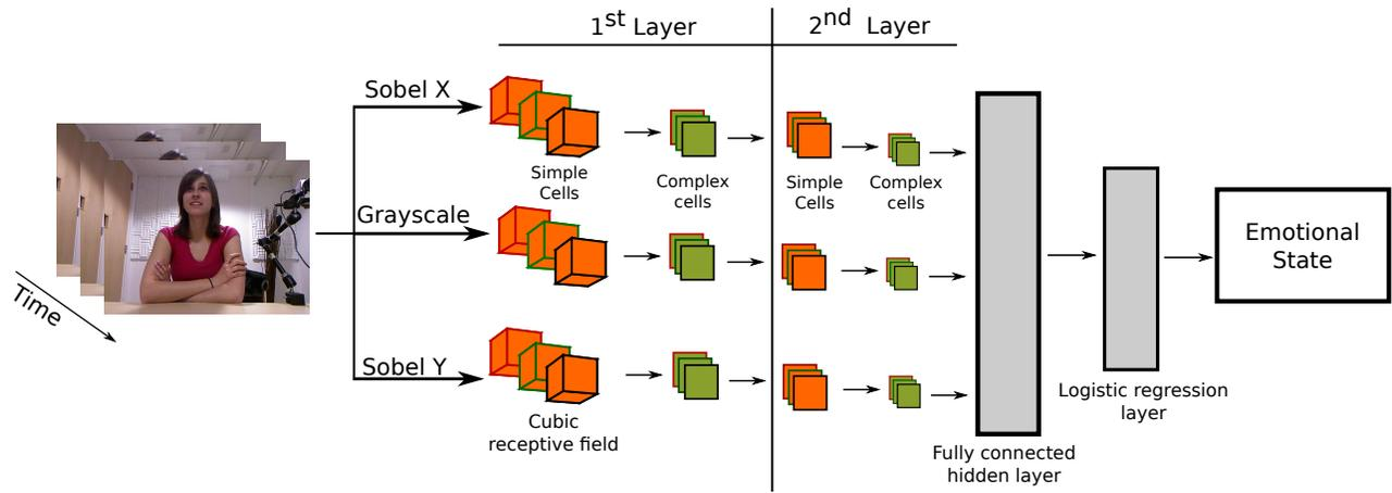
Fig. 3. Proposed architecture for a Multichannel Convolutional Neural Network using 3 channels and 2 layers. Two of the channels apply Sobel-like filters in each image of the sequence. In the first layer of each channel a cubic receptive field is implemented.
