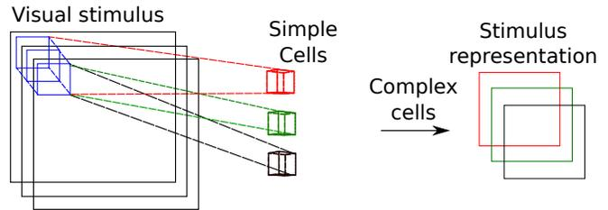
Fig. 2. Cubic receptive field implementation of the complex cells. Each filter implements a cubic kernel, which is applied to a stack of images, producing a single image which is applied to a pooling operator, simulating simple cells.
