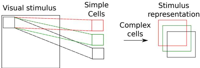
Fig. 1. Each layer of the CNN is composed of simple and complex cells, simulated using convolution and pooling operations. There are different filters representing simple cells that, when applied to the visual stimulus, generate a different representation. The pooling process reduces the dimensionality of the stimulus and increases the invariance of the representation.
