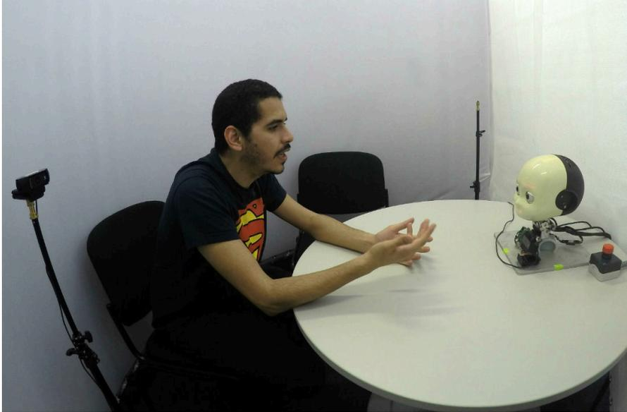
Figure 4.20: Picture of the HRI scenario. A person is seated in front of the iCub robot, which is the active subject.
