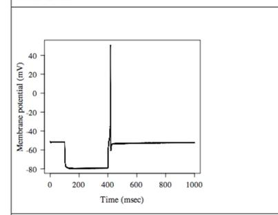
Figure 7. Rebound firing pattern, preliminary results. The Ca spike is generated by a standard T-channel. A T-channel with a longer time constant will probably be needed to produce the slower and more pronounced Ca spike seen *in vivo*.
